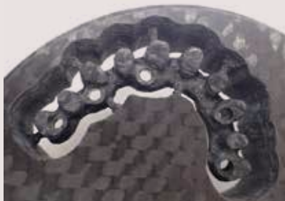
Fig 9. Carbon fiber framework milled from a disc
