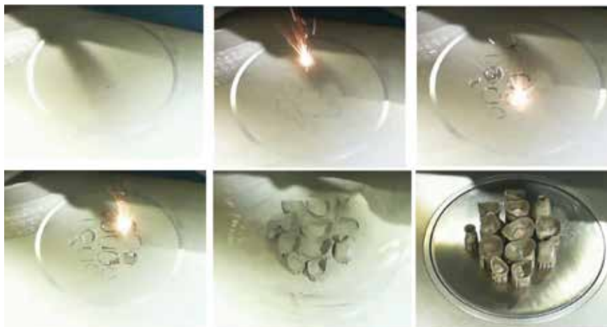
Fig 22 Laser sintering process. Moving laser beam melts each successive surface of metal powder until the metal crowns are fully formed
