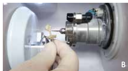
Fig 23 Chairside milling machines allow milling of single restorations, small bridges and surgical guides
