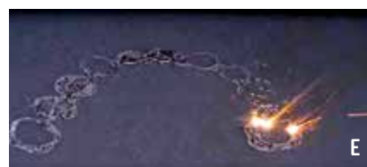
Fig 21 Laser sintering. (Selective laser sintering, selective laser melting, direct metal laser melting). The moving laser beam melts successive layers of metal powder converting them to a solid state. A roller rolls new powder layers for subsequent sintering as the crown or bridge is built up in layers
